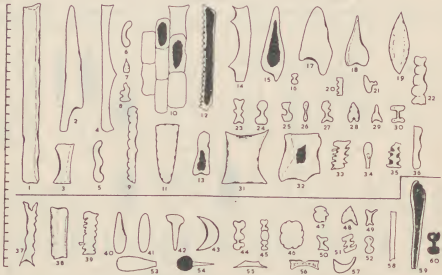
FIG. 9.—Sketches of outline shapes of opal-phytoliths in some Australian dusts. Nos. 1 to 36—from Mt. Isa, Q. (Table 1, No. 11), in dust from a collector placed 2 ft. above the ground and 3 yds. from the testing circuit track, on the down-wind side of a moving convoy of vehicles.
